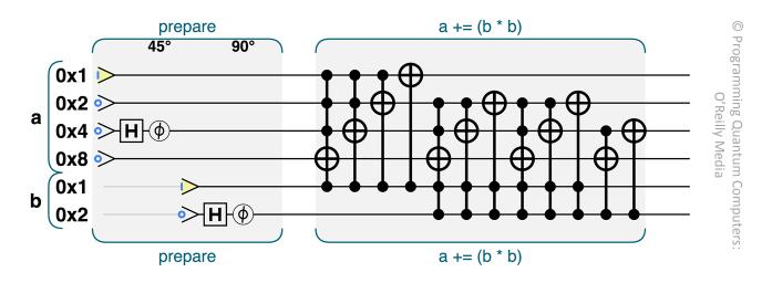
Multiplication by repeated addition, conditional on bits of *b*.
