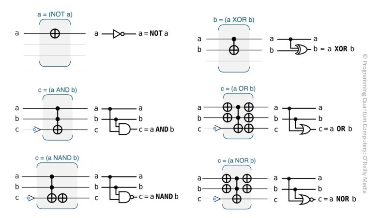
(Note the use of scratch qubits in the last four circuits)
